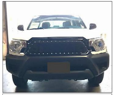
Step 4 Install grille onto vehicle by reversing steps 1-2 in the removal process.
