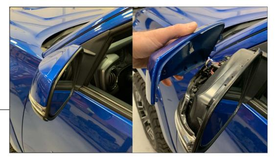
Carefully pull the mirror cover from the mirror. The cover is clipped onto the mirror. Firmly pull from the top edge and work around the mirror until it comes off.
