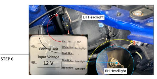
DRL Wiring: Using the supplied scotchlok connectors, connect the factory turn signals plugs to the control box wiring harness as follows:
