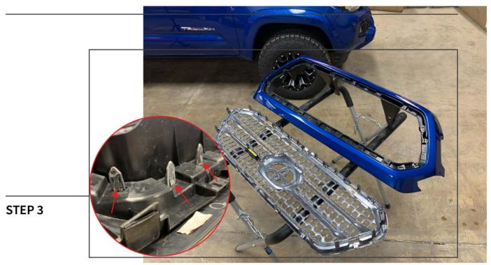
Using a flat blade screw driver, depress the grille insert tabs and remove the factory from the grille surround.
