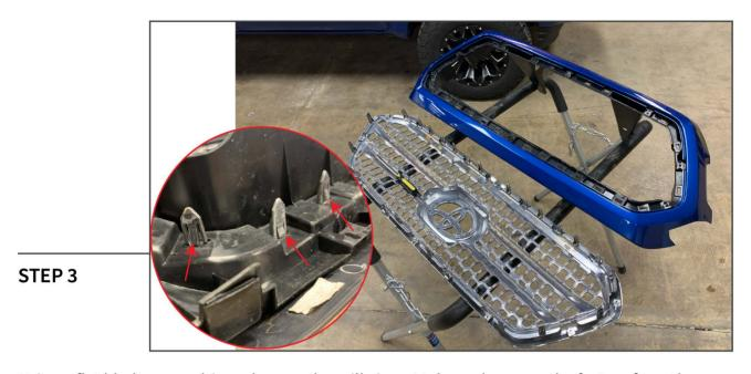
Using a flat blade screw driver, depress the grille insert tabs and remove the factory from the grille surround.
