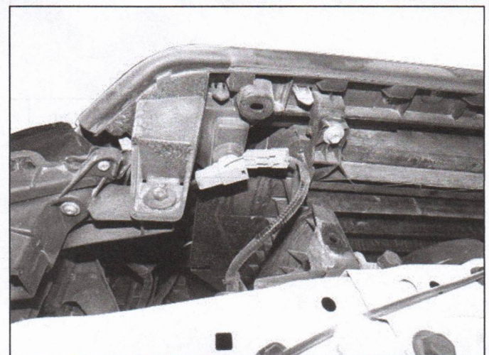
(Fig 12) Unplug driver side wire harnesses shown
