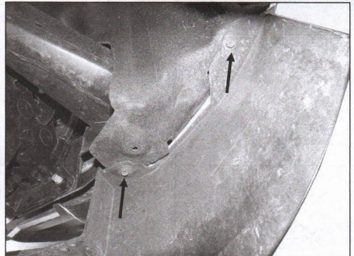
(Fig 4) Remove air dam from front clip by removing several screws from underneath on each side.
