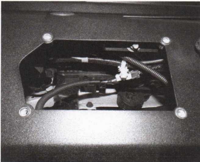
(Fig 62) Reach through the cutouts on each side of the Front Bumper Assembly and plug in the fog lights and front parking sensors using the Parking Sensor Extension Harnesses (if equipped)
