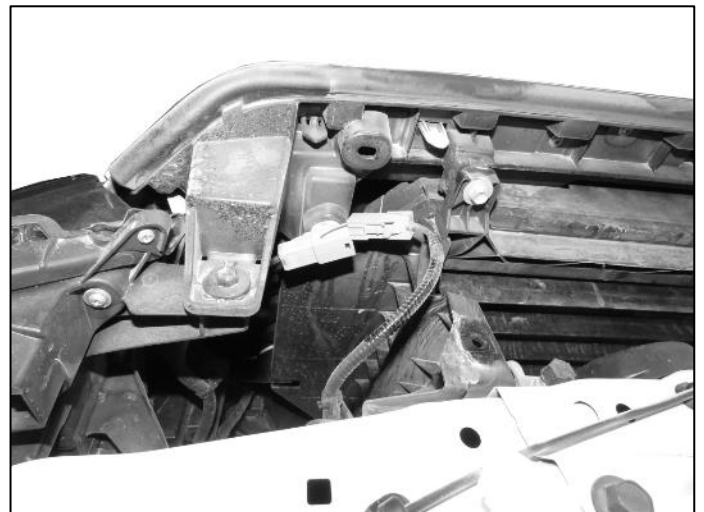
(Fig 12) Unplug driver side wire harnesses shown
