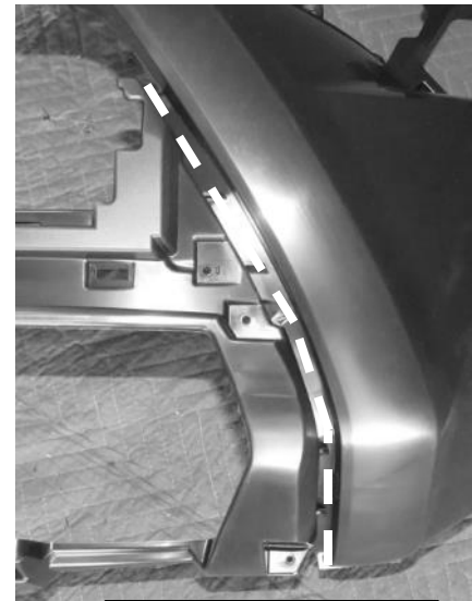
(Fig 37) Cut along the edge on the side of the front clip
