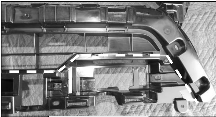
(Fig 33) Cut along the edge on the side and under the grille opening
