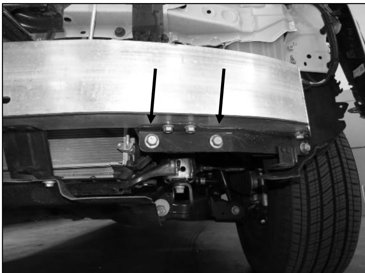
(Fig 17) Remove two lower frame horn bolts from crash bar. Repeat Steps 15-16 for Passenger Side, and fully remove crash bar.
