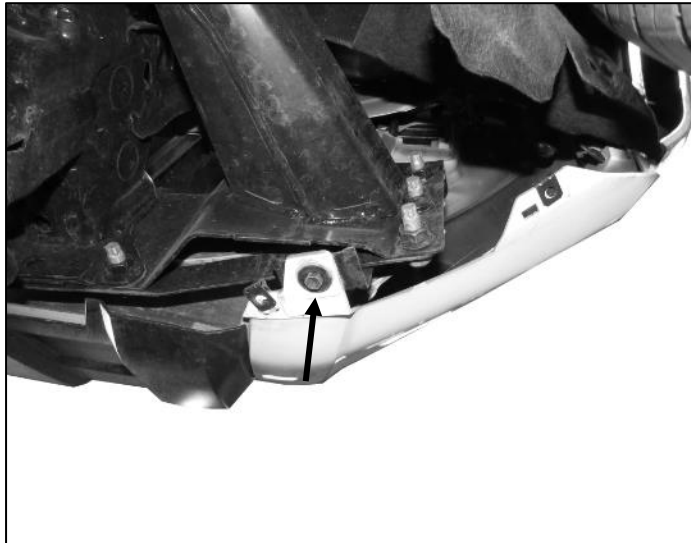
(Fig 7) Remove factory bolt to loosen side bottom section of front clip. Keep hardware in safe storage.
