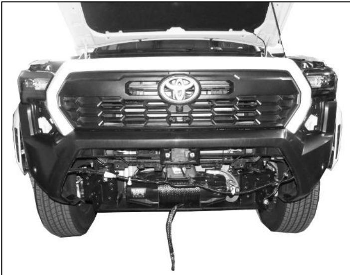
(Fig 50) Carefully reinstall the Front Clip onto the vehicle. Make sure all clips go into their original latch points and wire harness is not caught between any choking points.
