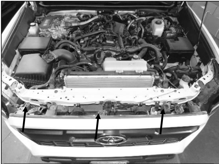
(Fig 9) After removing plastic covers and air intake, remove three bolts holding the upper clip.
