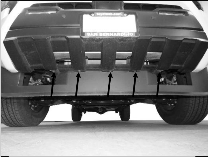
(Fig 5) Continue removing air dam by removing several screws from underneath at the center. Keep hardware in safe storage.
