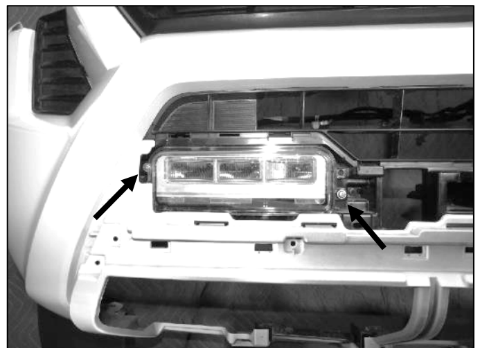
(Fig 31) From front side, remove fog lights.
