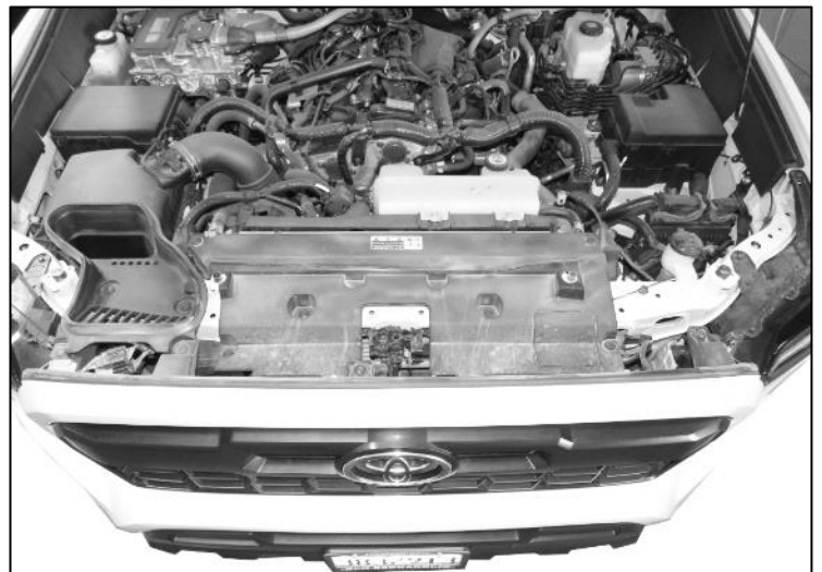
(Fig 8) Open the hood and remove plastic covers and air intake by unfastening clips and bolts. Plastic pry tool may help with removing plastic clips.
