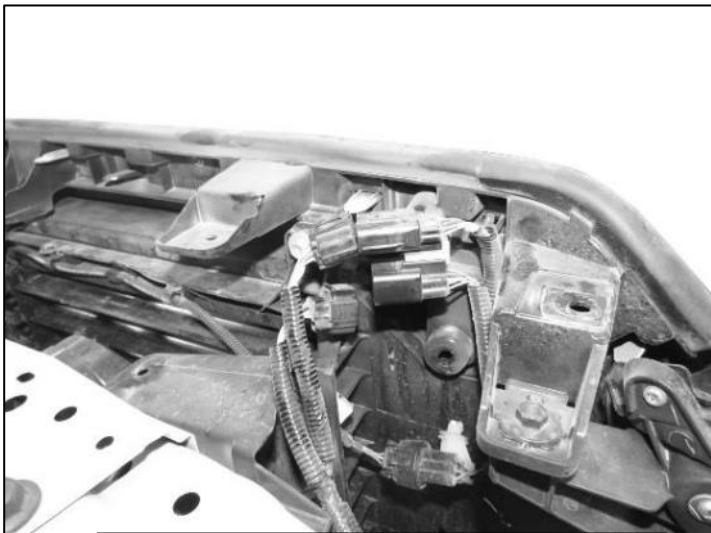
(Fig 11) Unplug passenger side wire harnesses shown
