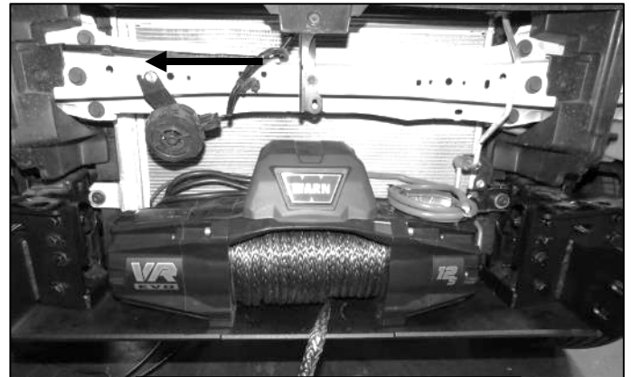
(Fig 48a) Hybrid Vehicles Only: Relocate pedestrian warning speaker if necessary
