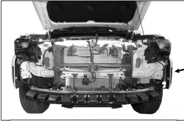
(Fig 13) Carefully release and pull the front clip off the vehicle and place it on a flat secure surface. Remove the plastic piece from the crash bar and place it aside.
