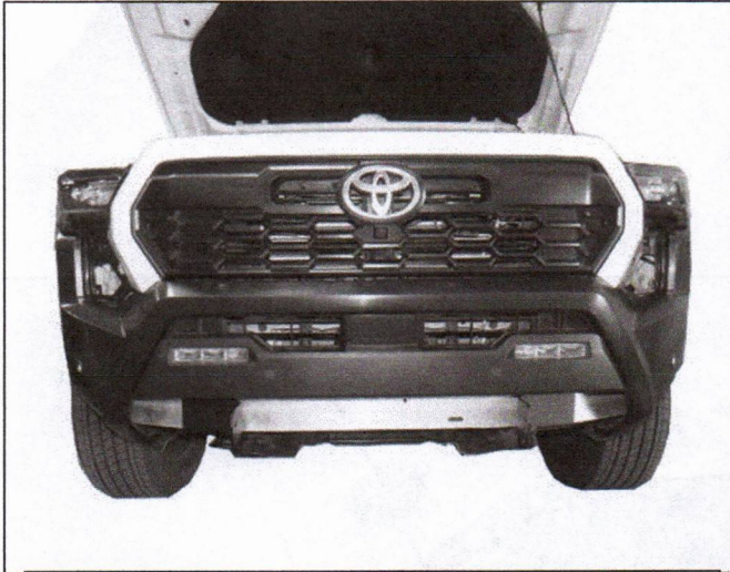
(Fig 26) Test fit the bumper and adjust any brackets for proper position before reinstalling front clip onto vehicle. The brackets will be difficult to adjust with the Front Clip on. When ready, refasten reinstall the Front Clip and all upper, side, and bottom screws and clips that were previously removed.
