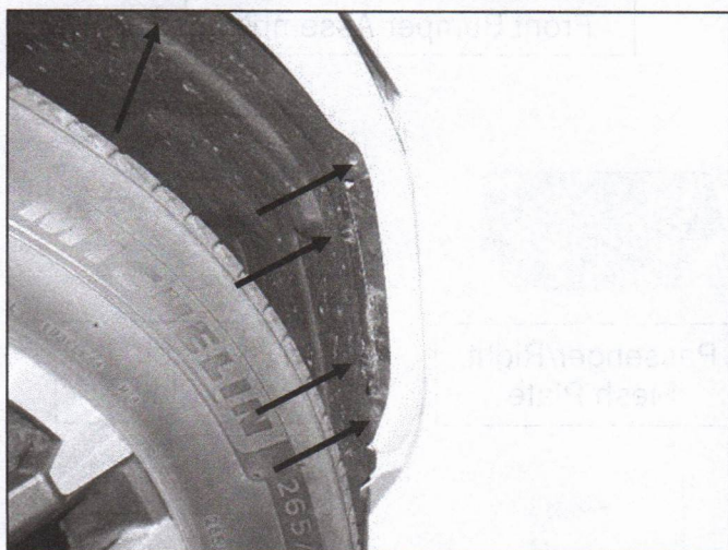
(Fig 1) Starting on Passenger Side wheel well, remove three screws and two plastic clips to release the liner from the front clip. Pry tool may help with separating liner from front clip. Repeat for Driver side. Be sure to retain all hardware.
