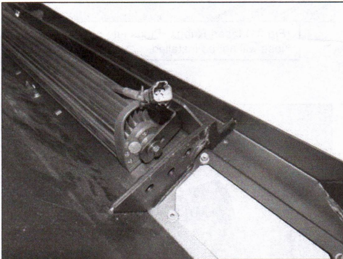
(Fig 28) Install LED light bar at center cut out at this time if using. Use LED Light Bar specific hardware to mount to bracket. Follow LED Light Bar's instructions to set up wiring to vehicle.
