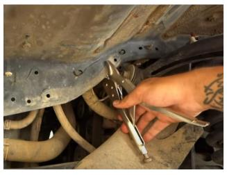
NOTE: To remove the Passenger Side bolt, gently push the A/C hard line out.
