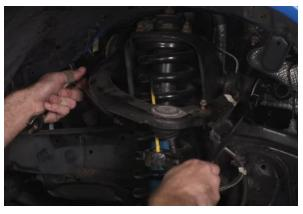
NOTE: To remove the Driver-side bolt, bend the pinch welded lip of the inner fender just enough to remove the upper control arm bolt completely.
