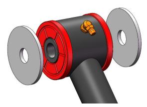
NOTE: Make sure that a washer is placed on each side of the bushings. Then, carefully feed the pivot bolt through the arm's pivots and through the pivot tube in the chassis, loosely securing the nut and washer.
