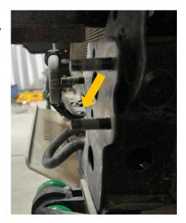
6. Lift the winch mount in place and secure using the factory bolts. Make sure to connect the motor ground and control box ground to the winch before bolting the winch down because it is difficult to read once bolted down. Use the rear 2 winch bolts to install the lower valance bracket.
