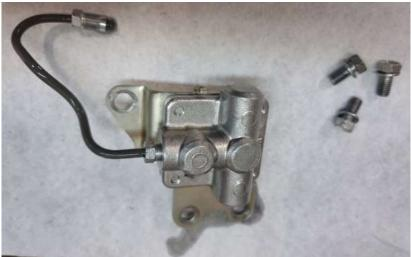
Install the new supplied Stainless Line as shown.
