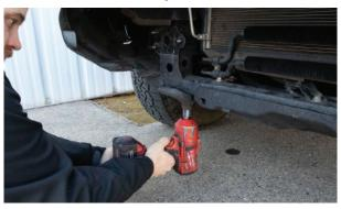
**9.** Remove the (2) screws securing the sub frame extensions to the frame. Keep the sub frame extensions in place.
