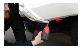
**6.** Remove the (6) nuts holding the aluminum crash bar to the standoffs. Remove the crash bar from the vehicle by angling it out of the hole you cut in the center of the bumper.
