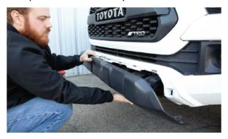
**3.** Remove the front plastic crash structure by unclipping it from the aluminum crash bar.
