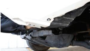
**13.** Mount the winch plate onto the frame as shown using the original crash bar mounting nuts. Initially position the frame studs in the center of the slotted holes in the winch plate. Snug up a few of the nuts to hold the winch plate in place.
