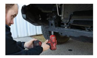
**10.** Unbolt the transmission cooler from the frame crossmember and relocate it rearward using the provided relocation brackets and hardware.
