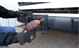
**2.** Remove the front bumper trim piece by prying it forward, away from the bumper. If you plan on reusing the trim piece, be careful not to break the plastic clips that hold the trim piece onto the bumper.
