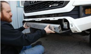
7. Remove the (6) nuts holding the aluminum standoffs to the frame.
