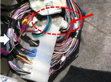
On the white connector, identify the Teal and White wires. Connect the High and Low wires from the main harness (J) using the supplied wire taps (L). After successfully connecting the wires, return the connector back into its place and check that it is secure.
