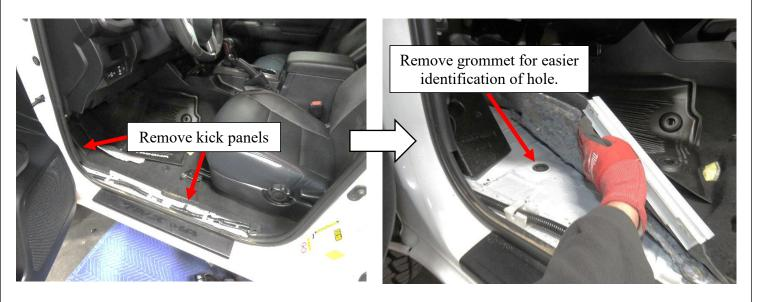
On the underside of the driver side, locate and remove the floor grommet in the floor panel above the frame. The grommet will be in a tight space above the frame and OE conduit. Poke a hole through the grommet and thread the two signal wires through and up into the vehicle cabin.
