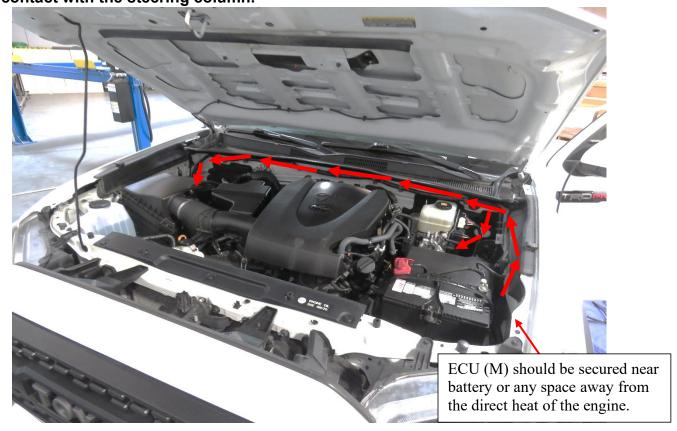
Route the shorter (marked "Passenger-side") leg of the harness down the Passenger-side wheel well. **Be sure to avoid contact with any moving or hot engine components.** Attach and secure the main harness (J) with supplied cable ties.
