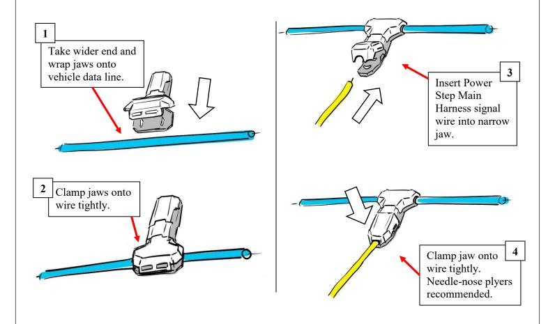
NOTE: Make sure wire is seated properly in the jaws before clamping. The wire being tapped must be centered on the "teeth" to make a proper tap.
