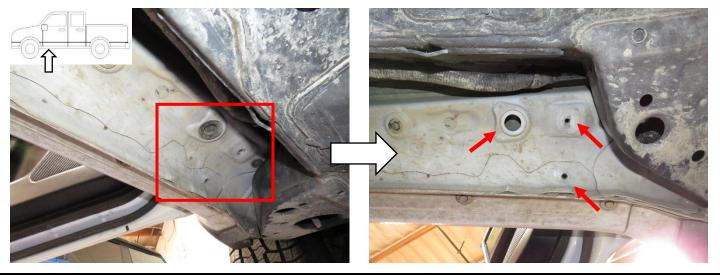
Next, take a Large Bolt Plate (O) and insert it into the large hole where the rubber plug was. Once the bolt plate sits in the hole with the threaded end stick out, use a Plastic Insulator to help the Large Bolt Plate stay in place.
