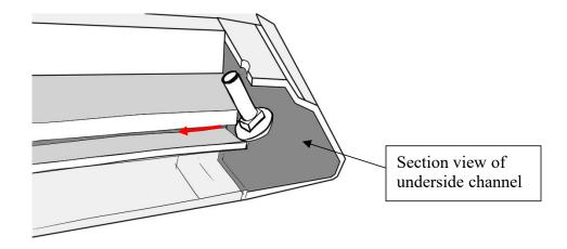
Perform a function check by closing the driver side front door and opening it again. The front bracket assembly (A) motor should activate the linkage arm and move it into the down or "deployed" position.
