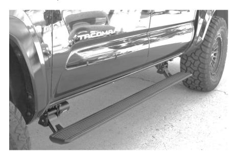
\*NOTE: If board does not move during troubleshooting, check the tapped CAN Signal High and Low wires.
