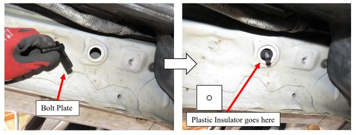
Locate Driver Side rear mounting points on the rocker panel. Remove the OE bolts before mounting the rear bracket.
