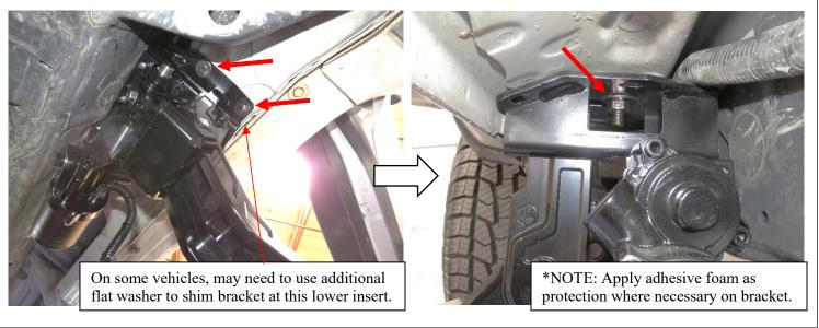
Locate rear mounting points. Next, line up rear mounting bracket slots to the threaded inserts and place Driver Side/Left Rear Bracket Assembly (B) onto rocker panel. Then fasten Hex Bolts (H), Lock Washers (I), and Flat washers (G). Do not tighten all the way yet.
