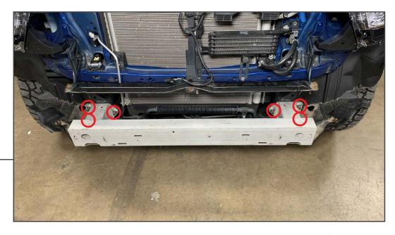
Remove (6) 14mm nuts from the aluminum bumper bar, and remove the bumper bar from the vehicle. The OEM (6) 14mm nuts will be reused.
