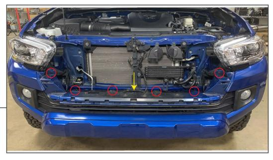
Remove (6) push clips from the bumper. Unplug the connector in the middle of the bumper.
