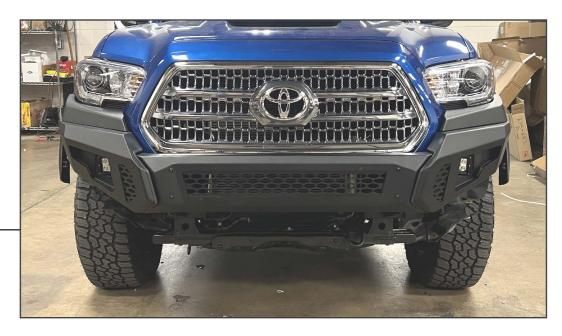
With a helper, lift the bumper to the previously installed mounting brackets. Loosely secure the bumper to the brackets using (6) M10 x 40mm bolts, (6) M10 lock washers, (12) M10 flat washers [24mm OD], and (6) M10 nuts.
