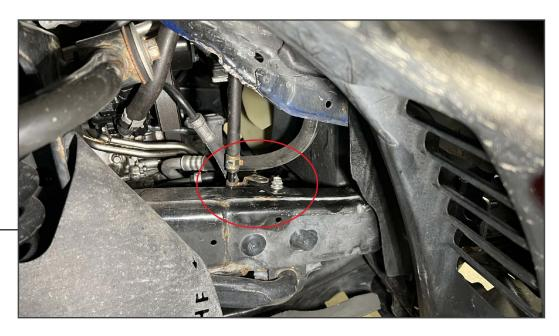
Power Steering Cooler Relocation (cont.): Through the RH side wheel well, remove the rubber liner covering the engine bay components. Unbolt the power steering cooler line from the frame. Then, fit the (1) line bracket between the cooler line and the vehicle frame. Use the original 12mm bolt to secure the bracket to the frame, and the included (1) M8 x 25mm bolt, (2) M8 flat washers [16mm OD], and (1) M8 lock nut through the cooler line bracket.
