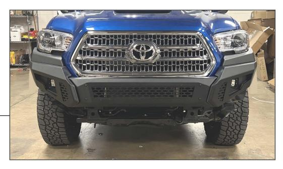
Verify all hardware is fully tightened. Ensure fender liners and fender flares are secure to vehicle.
