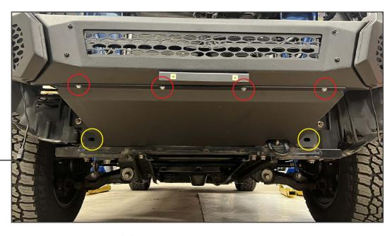
Install the skid plate to the bumper using (4) M6 x 20mm Allen combo bolts. Then, secure the skid plate to the vehicle frame using (2) M12 x 120mm bolts, (4) M12 flat washers, and (2) M12 lock nuts. Adjust the skid plate to the vehicle, and tighten all hardware.
