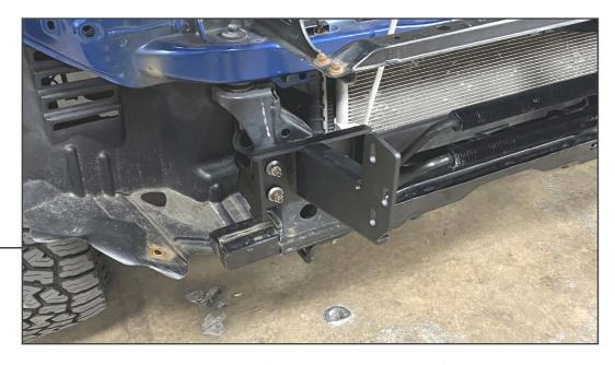
Fit the LH and RH mounting brackets to the vehicle frame using the original (6) 14mm nuts. Do not fully tighten the brackets at this time to allow for adjustments later.
