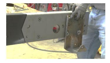
Then, take your leaf spring hangers bracket and hold it up to the leaf spring hanger under your frame rail. Insert the two remaining bolts and nuts and screw them in with a 14mm socket and 15mm wrench.
