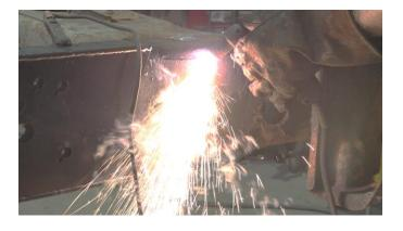
Remove the rivets retaining your rear leaf spring hanger and its bracket.
