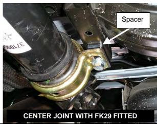
Tighten both bolts firmly.
