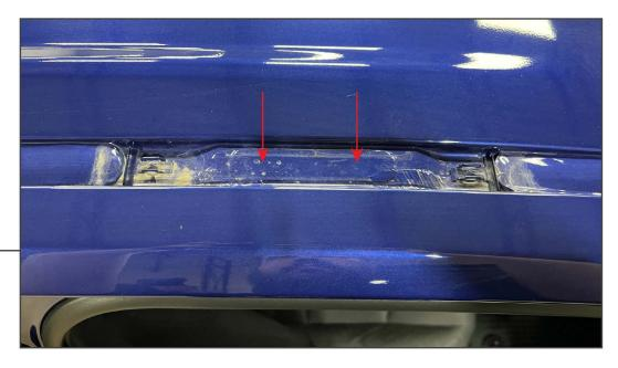
Under the plastic cover is painted double sided tape. Press the tape downwards to locate the bolt holes under the tape.
