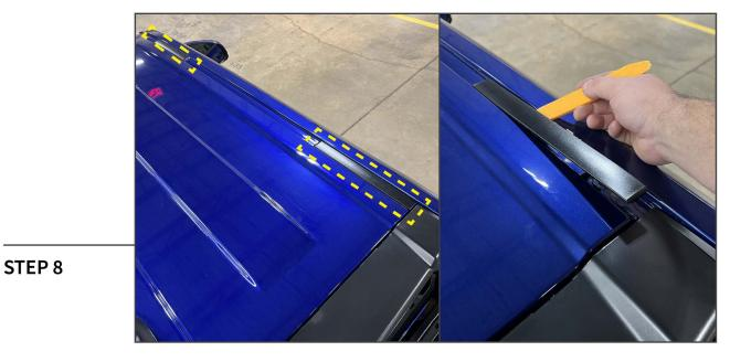
Above the vehicle doors along on the roof, locate the (2) plastic covers per side. Using a plastic panel removal tool, lift the covers away from the vehicle.
