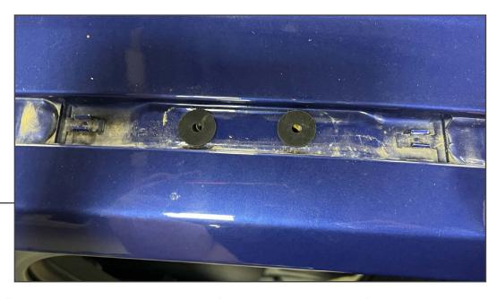
Place (1) rubber flat washer around each vehicle roof bolt hole. Then, place (1) 7mm spacer on top of the rubber flat washers.
