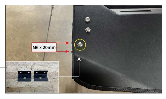
Fit (1) "L" bracket behind the front panel, and secure using (2) M6 x 20mm Allen bolts, (4) M6 flat washers, and (2) M6 lock nuts to the side rail. Then, secure the "L" bracket to the front panel using (1) M8 x 25mm Allen bolt, (2) M8 flat washers, and (1) M8 lock nut.
