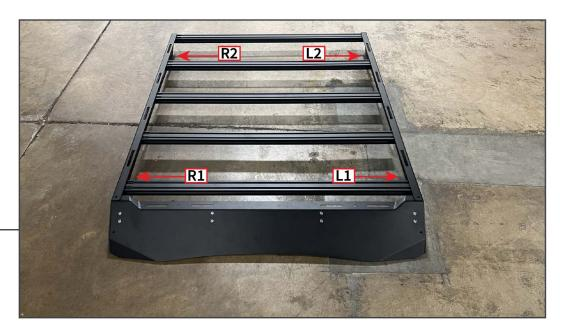
Identify the included mounting brackets using the diagram above. Mount the appropriate mounting braket to the inside of the side rails using (2) M8 x 25mm Allen bolts, (4) M8 flat washers, and (2) M8 lock nuts per bracket. The brackets will face inwards on the roof rack.
