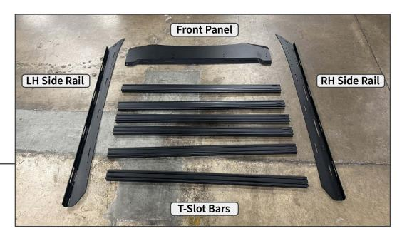
Lay out and identify all roof rack components.
