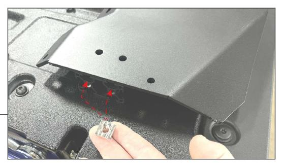
With the remaining (1) T-Slot bar, place the bar on a workable surface with the rectangular T-Slot opening facing down. Then, slide the included (8) T-Slot nuts into the end of the T-Slot bar and route each T-Slot nut to the (8) bolt holes in the front panel. Secure the T-Slot bar to the front panel using (8) M8 x 16mm Allen bolts, (8) M8 lock washers, and (8) M8 flat washers.
