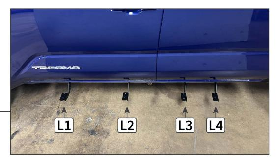
Loosely install the included mounting brackets to the vehicle chassis threaded holes using the included (8) M8 x 20mm bolts, (8) M8 lock washers, and (8) M8 flat washers.
