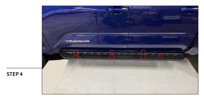
Remove the pre-installed M6 hardware from the side step mounting studs.
