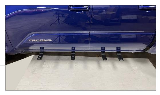
Loosely install the included mounting brackets to the vehicle chassis threaded holes using the included (6) M8 x 20mm bolts.
