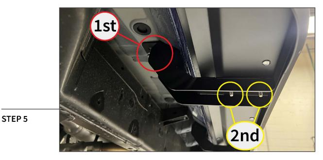
Adjust the side steps & bracket as necessary for best fit, then tighten the mounting hardware to secure into place using the diagram above.
