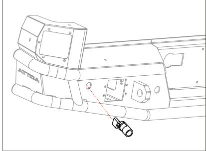
**Step 3:** Attach the blind sensor housing to the bumper.
