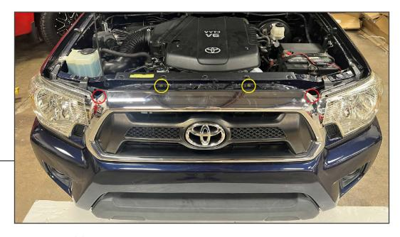
Remove (2) 10mm screws and (2) plastic push clips from the top of the grille. Lift the center tabs, and remove the grille from the vehicle.
