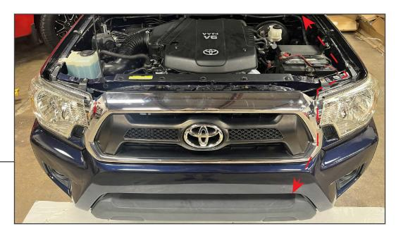
Carefully route the wiring harness across the vehicle.
