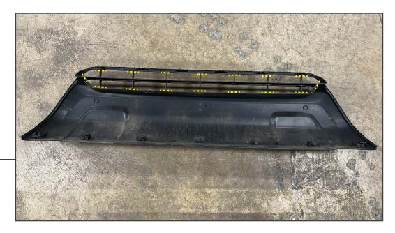
**2005-2011 vehicles:** Trim the grille section of the lower trim panel to allow light bar clearance.
