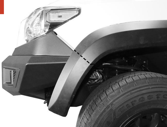
(Fig 23) Cut fender flare to match end of Bumper
