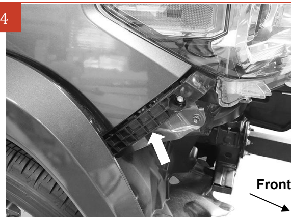
(Fig 4) Remove plastic block (arrow) from front edge of fender (passenger/right side pictured)
