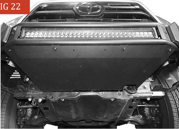
(Fig 22) Splash Guard installed
