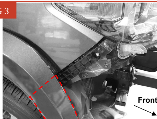
(Fig 3) Release the front leading end of the fender flares (Dashed line area) from the bumper cover
