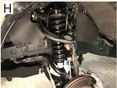
\*\*4 Wheel Alignment is highly recommended after completion to prevent premature tire wear\*\*
