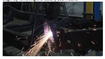
Grind the work area free of rust and debris, revealing bare metal/ followed by coating the work area with a weld through primer to help prevent against further rust development.
