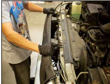
Pull up on radiator grill to pop out then remove and set grill aside.
