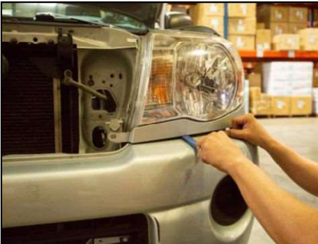
Use panel popper under headlight trim to release tab and remove trim. Repeat on other side.
