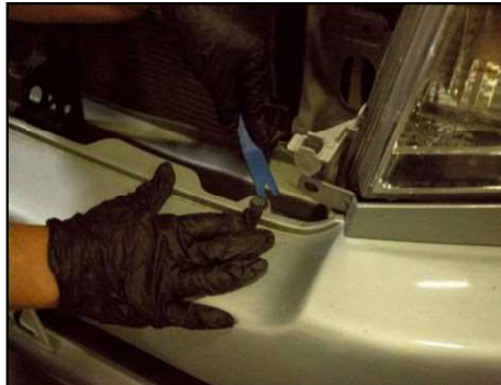
Remove 3 push tabs from top of bumper.
