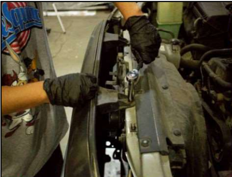
Remove two 10mm bolts from top of grill.
