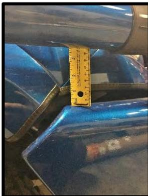
35. **CRITICAL:** Set distance from top face of the bull bar wing to bottom of rail to 85mm +/- 2mm for correct set up.
