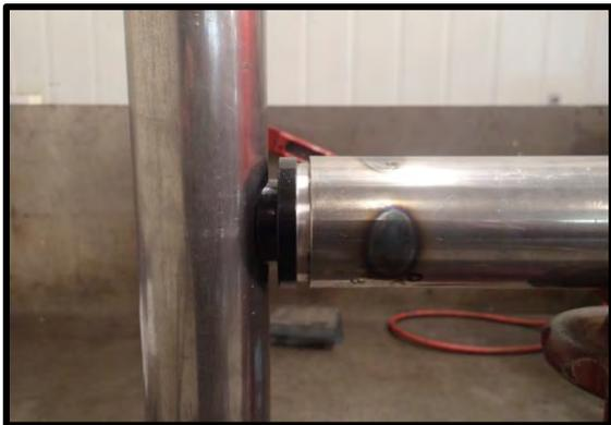
33. Hold Side Rail so that when viewed from the side of the vehicle the top tube runs parallel to the installed Side Steps and the Side Rail sits as desired against the side of the vehicle.
