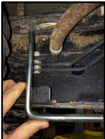
12. At the marked off locations on the driver side rail, insert the U-bolts upward between the wire harnesses and frame rail, as shown in the diagram, and then pivot the bolt so the threads point outwards.
