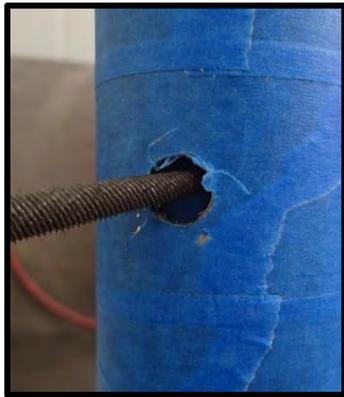
53. Using a small flat or half-round file carefully remove any burrs from the edge of the Ø12mm hole.
