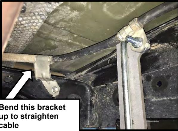
26. Re-locate the handbrake cable bracket previously on the top of the frame rail onto the corresponding load plate using the supplied M8 x 25 hex bolt and M8 nyloc nut. Stack (3) M8 Flat washers in between the load plate and hand brake bracket as shown in the diagram. Slightly bend the near handbrake bracket located on the crossmember to straighten the cable out as much as possible.
