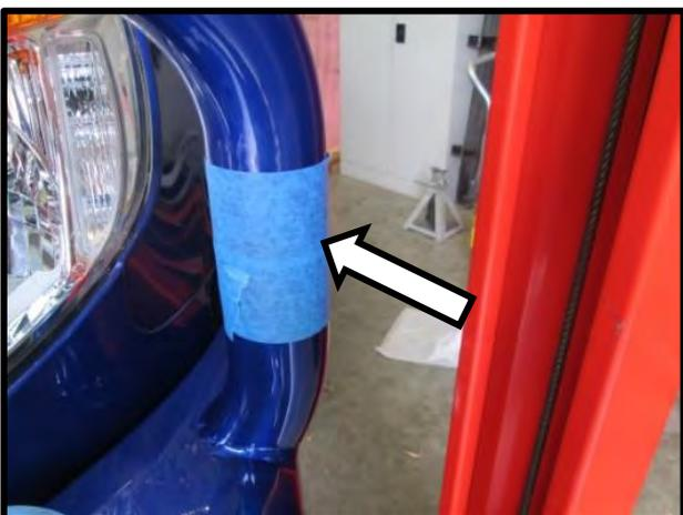
29. Use masking tape to wrap **1 x layer only** of tape around the Bull Bar Outer Frame to protect it from damage. Ensure masking tape is applied flat and without creases.
