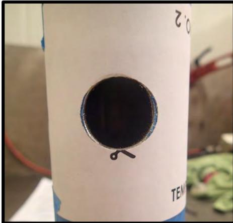
48. Carefully align "TEMPLATE 2" and center over the Ø24mm hole. Wrap around the outer frame tube.
