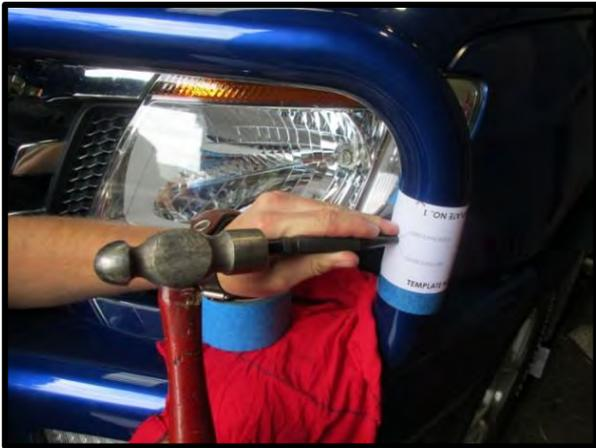
**Important:** Cover the upper surfaces of the bulbar wing with masking tape of rags to prevent damage from drill swarf.
