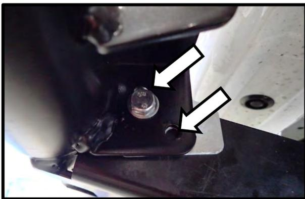
58. Tighten M8 bolt connecting the front rail to the step section ensuring the slot and holes in the spacers (if fitted) are aligned with the holes in the step sections and front rail.
