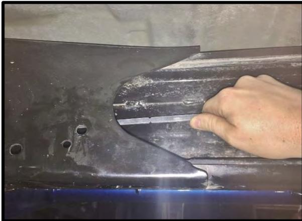
17. Insert the M12 x 1.75 cage nut in the front mount support nut plates.
