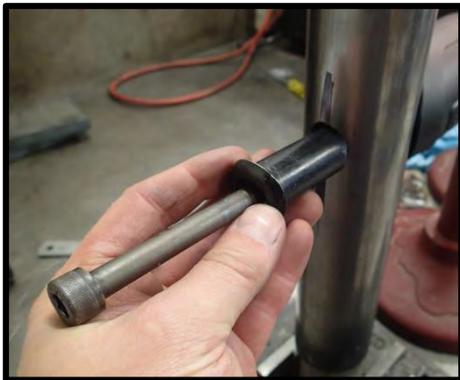
57. Install submerged bushing and M10 socket head cap screw.
