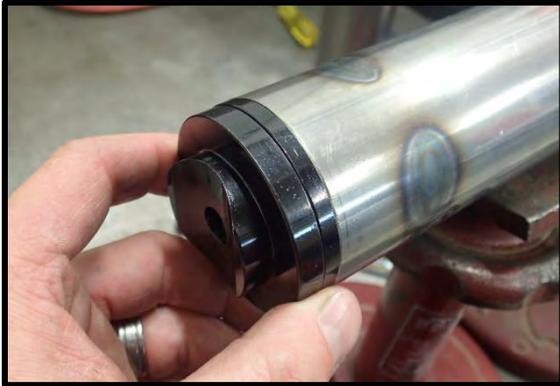
37. Swing the Side Rail outwards and away from the vehicle allowing installation of appropriate/selected spacer into gap between the front end of the Side Rail and the tube spigot. (5mm shown in this instance).
