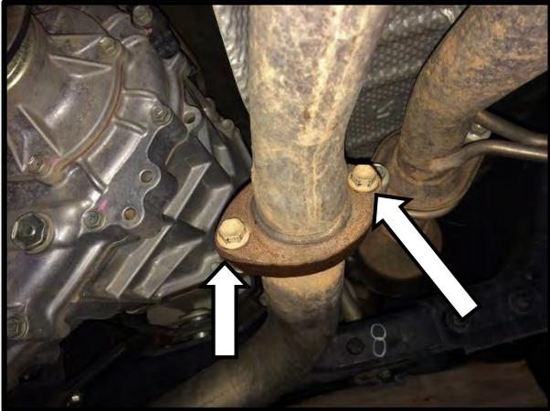
9. In order to reinstall the cross member through bolts in the correct orientation, it is necessary to loosen the section of the exhaust piping in that area.
