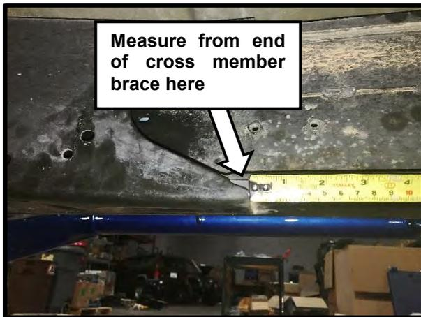
4. **Starting with the driver (left) side**, mark out 233mm and 765mm from the cross member brace, as shown, on the frame.
