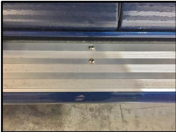
67. Run a bead of silicon along the top of the rail where the tread plate will sit. (This will help prevent vibration).
