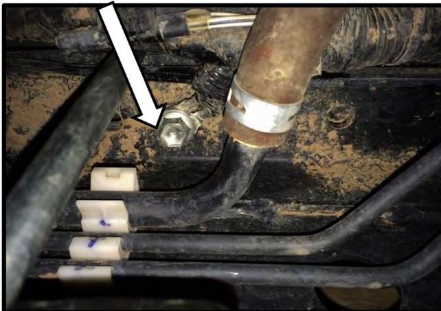
6. At the 765mm location on the driver side it is necessary to relocate the ground cable bolted to the top of the frame. Remove the hex screw and ground wire eyelet and reinstall on the opposite side of the frame using the same weld nut.
