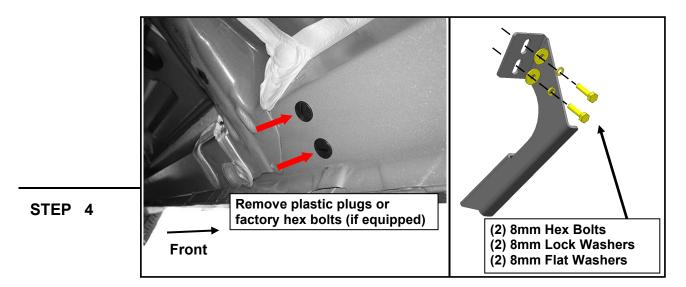
Remove the plastic plugs or hex bolts. Loosely fit the (1) Driver Center bracket to the vehicle threaded body hole using (2) M8 x 30mm bolts, (2) M8 lock washers, and (2) M8 flat washers. Do not fully tighten to allow for later adjustments. Repeat this step for the Driver Rear bracket.
