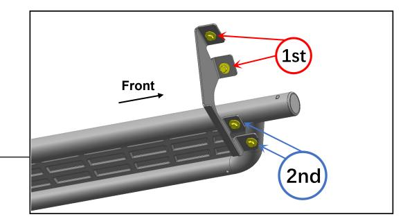
Tighten the mounting brackets to the vehicle. Adjust the running board to the desired angle, and tighten the M8 combo bolts to secure the step into place. See photo for tightening order visual.
