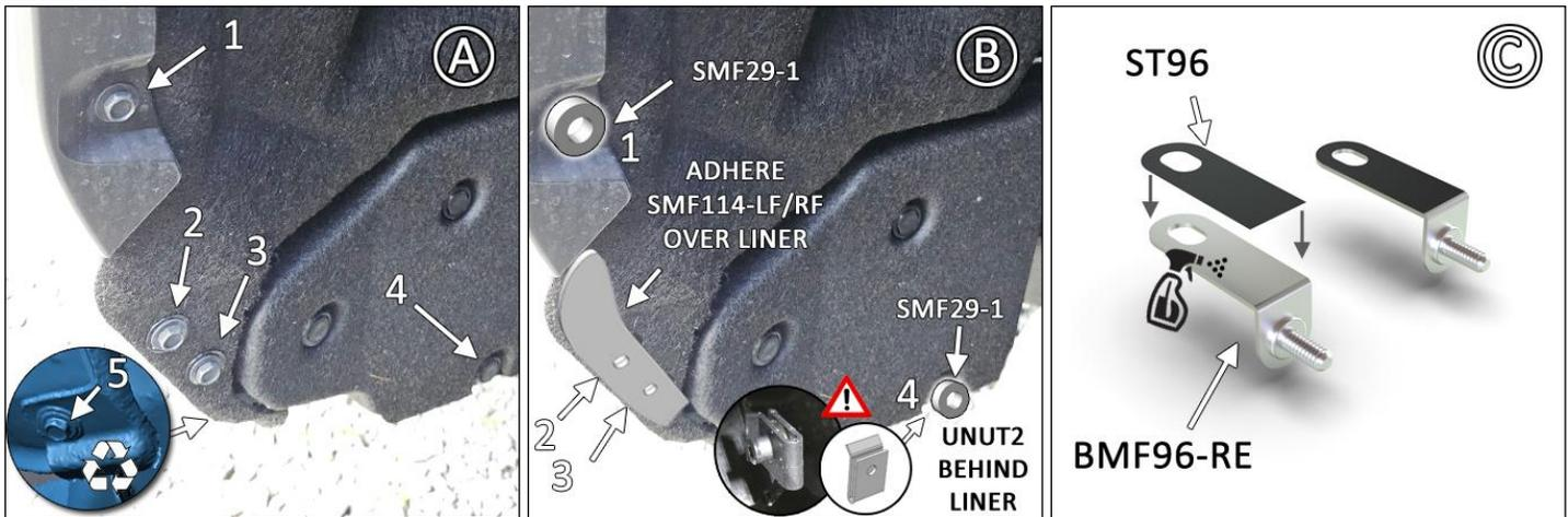
**IMAGE D** Place BMF96-RE over mount 5, then reinstall fastener 5.
