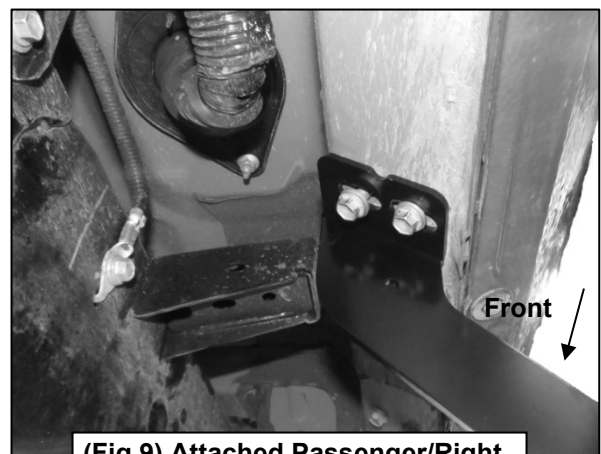
(Fig 9) Attached Passenger/Right Rear Mounting Bracket
