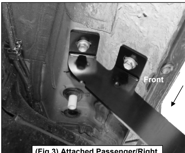
(Fig 3) Attached Passenger/Right Front Mounting Bracket
