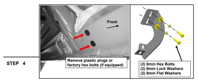
Remove the plastic plugs or hex bolts. Loosely fit the (1) Driver Center bracket to the vehicle threaded body hole using (2) M8 x 30mm bolts, (2) M8 lock washers, and (2) M8 flat washers. Do not fully tighten to allow for later adjustments. Repeat this step for the Driver Rear brackets.
