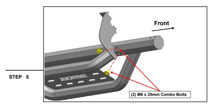
With all brackets loosely mounted to the vehicle, fit the running board onto the brackets, and loosely secure into place using (6) M8 x 25mm combo bolts.
