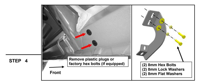
Remove the plastic plugs or hex bolts. Loosely fit the (1) Driver Center bracket to the vehicle threaded body hole using (2) M8 x 30mm bolts, (2) M8 lock washers, and (2) M8 flat washers. Do not fully tighten to allow for later adjustments. Repeat this step for the Driver Rear bracket.
