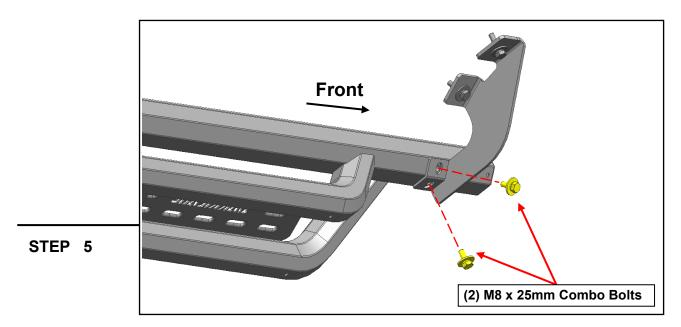
With all brackets loosely mounted to the vehicle, fit the drop step onto the brackets, and loosely secure into place using (6) M8 x 25mm combo bolts.
