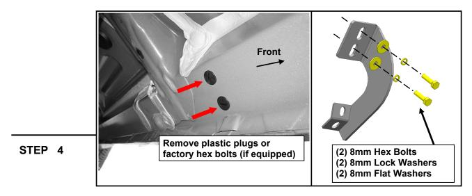
Remove the plastic plugs or hex bolts. Loosely fit the (1) Driver Center bracket to the vehicle threaded body hole using (2) M8 x 30mm bolts, (2) M8 lock washers, and (2) M8 flat washers. Do not fully tighten to allow for later adjustments. Repeat this step for the Driver Rear brackets.
