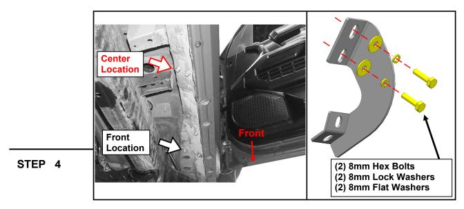
Loosely fit the (1) Driver Center bracket to the vehicle threaded body hole using (2) M8 x 30mm bolt, (2) M8 lock washer, and (2) M8 flat washer. Do not fully tighten to allow for later adjustments. Repeat this step for the Driver Rear bracket.
