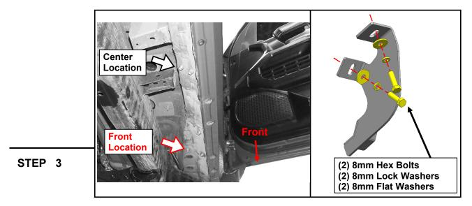
Start installation toward the front of the Driver/Left side of the vehicle.
