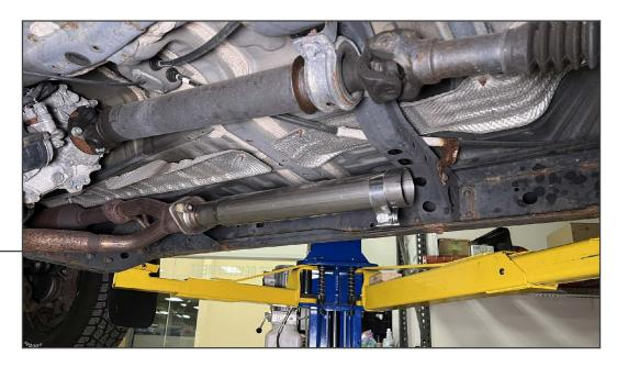
Ensure the exhaust gasket is in place on the vehicle exhaust pipe. Fit the front pipe to the vehicle exhaust pipe, and loosely secure using the OEM (2) 14mm spring bolts.
