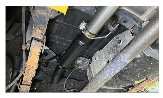
Fit the muffler w/ turn down onto the intermediate pipe, and loosely secure using the previously placed 3" hanger clamp. Secure the muffler assembly to the (2) OEM vehicle rubber hangers.
