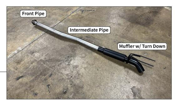
Lay out and identify all exhaust components.
