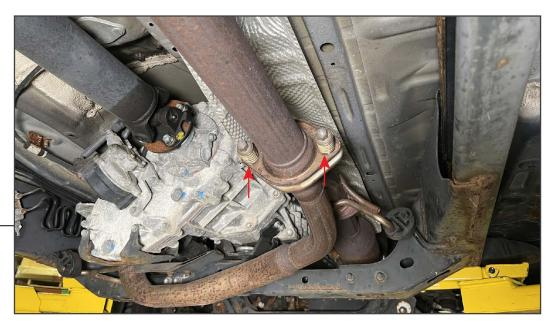
Safely lift and support the vehicle off the ground using a floor jack and jack stands. Locate the vehicle exhaust flange towards the front of the vehicle. Remove (2) 14mm spring bolts from the exhaust flange.
