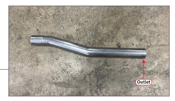
For <u>Double Cab Short Bed</u> OR <u>Access Cab</u> Vehicles [128in Wheelbase]: Cut 13" from the outlet side of the intermediate pipe.
