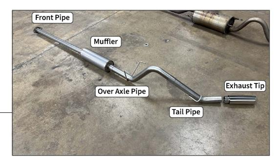
Lay out and identify all exhaust components.
