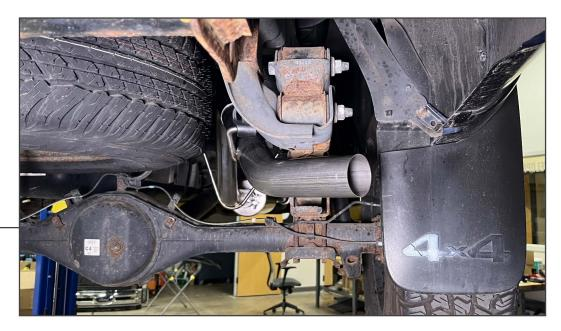
Fit the (1) tail pipe into the over axle pipe, and loosely secure using the previously placed (1) 3" exhaust clamp. Fit the tail pipe into the previously placed rubber hanger.
