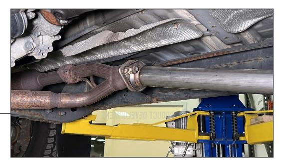
Ensure the exhaust gasket is in place on the vehicle exhaust pipe. Fit the front pipe to the vehicle exhaust pipe, and loosely secure using the OEM (2) 14mm spring bolts.
