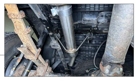
Fit the (1) over axle pipe into the muffler and into the (2) vehicle rubber exhaust hangers.
