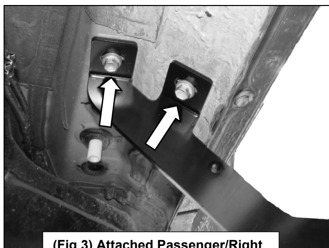
(Fig 3) Attached Passenger/Right Front Mounting Bracket at Front Mounting Location
