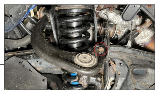
Remove (1) 10mm bolt from the ABS line retainer. Remove the line retainer from the control arm.
