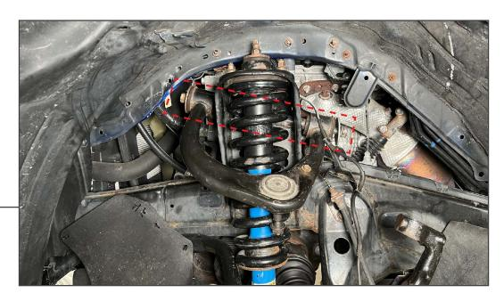
The vehicle uses (1) through-bolt through the vehicle frame to secure both ends of the control arm.
