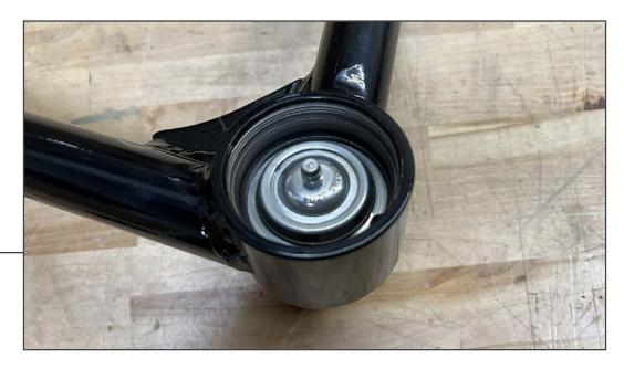
Turn the ball joint cap counter-clockwise to remove the ball joint cap to reveal the grease fitting. Fill the ball joint with synthetic grease until full, do not overfill.
