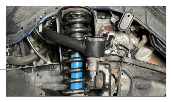
Secure the control arm ball joint to the vehicle steering knuckle using the (1) 19mm lock nut.
