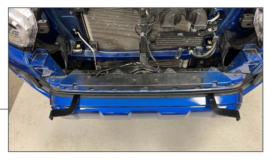
Route the flat side of the upper mounting brackets through the bottom outer-most slot in the vehicle bumper on each side. Secure each mounting bracket to the previously mounted stud plates using (1) M10 flat washer, (1) M10 lock washer, and (1) M10 nut per bracket. Ensure the stud plate is not touching the radiator fins while tightening the bracket into place.
