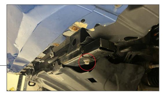
Remove (1) 17mm bolt from the frame rail extension panel.
