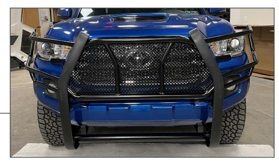
Adjust the grille guard to best fit the vehicle. Once properly adjusted, tighten all hardware evenly until secure.
