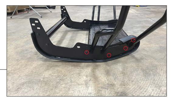
Fit the center grille guard panel in between the LH and RH bumper panels. Then, align each headlight guard to the center grille guard panel and the bumper panels. Once aligned, loosely secure the panels together using (8) M8 x 40mm bolts, (16) M8 flat washers, and (8) M8 lock nuts.
