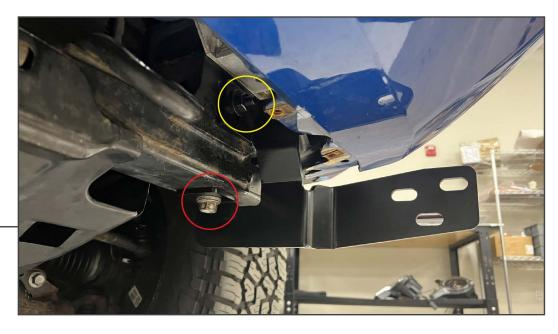
Fit the lower mounting bracket to the previously mounted stud plate. Then, loosely secure to the stud plate using (1) M10 flat washer, (1) M10 lock washer, and (1) M10 nut.
