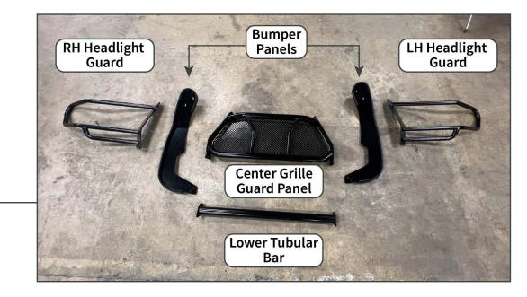
Lay out and identify all grille guard components on a soft workable surface.
