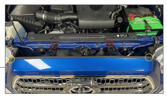
Open the vehicle hood. Remove (2) 10mm screws and (2) plastic push clips from the top of the grille. Then, pull the grille away from the vehicle to remove the grille from the vehicle.
