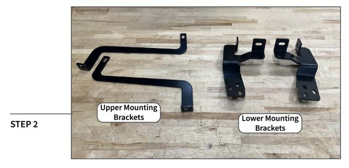
Lay out and identify all grille guard mounting brackets and hardware on a workable surface.
