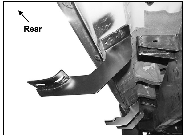
(Fig 6) Driver/left rear Mounting Bracket installed
