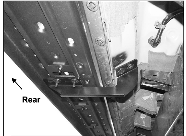
(Fig 10) (Fig 7) Driver/left Running Board attached to Rear Mounting Bracket
