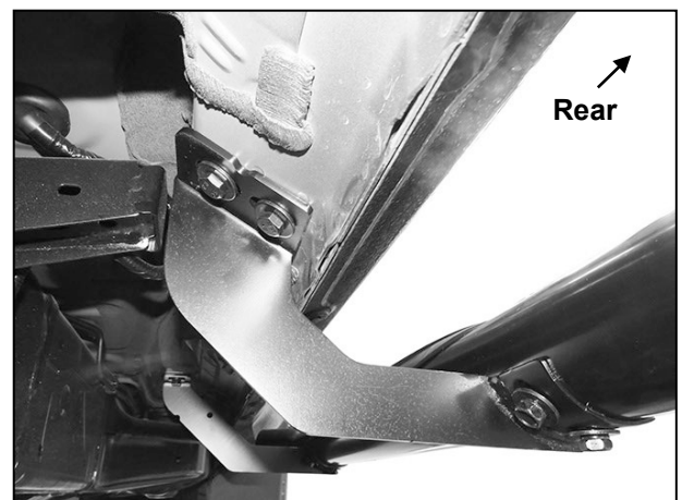
(Fig 7) Passenger/right Side Bar attached to Front and Center Mounting Brackets
