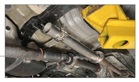
Fit the front pipe to the vehicle exhaust system using the original (2) 14mm bolts. Ensure the pipe bend is angled upwards. Then, fit (1) clamp hanger onto the end of the front pipe. Insert the hanger clamp through the rubber hanger from the rear towards the front of the vehicle.
