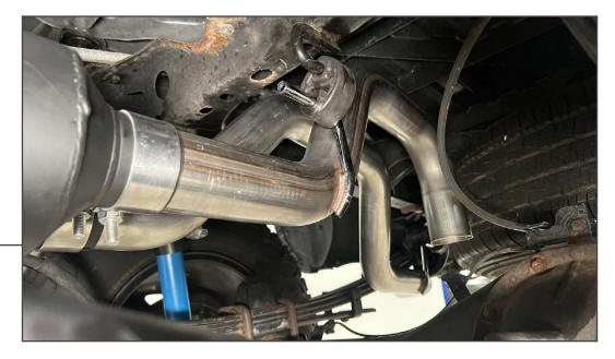
Fit the LH over axle pipe into the muffler, and fit the pipe hanger into the vehicle rubber hanger. Loosely secure the over axle pipe to the muffler using the previously placed 2.5" exhaust clamp.
