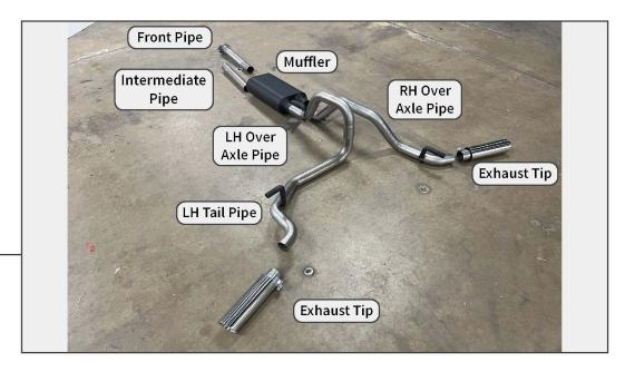
Lay out and identify all exhaust components.
