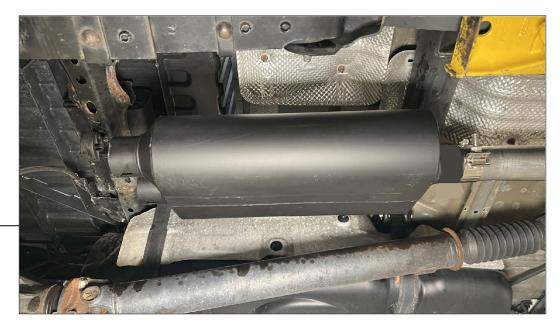
Fit the muffler onto the previously installed front pipe(s). Then, loosely secure the muffler using the hanger clamp.
