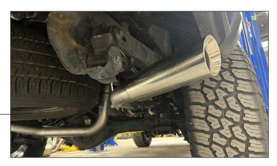
Lower the vehicle to the ground to apply weight to the vehicle suspension. Fit the (2) exhaust tips to the exhaust system.
