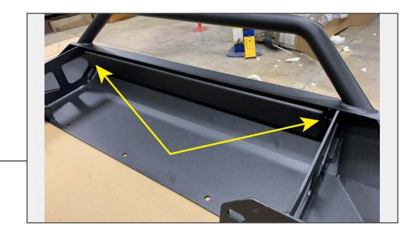
**Optional LED Light Bar:** Remove the M6 hardware to remove light bar block off plate prior to installing light bar.
