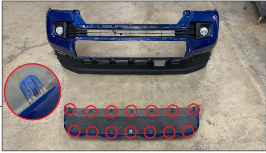
Remove the center panel in the bumper using a flathead screwdriver, and depressing the locking tabs. Remove the panel through the face of the bumper.
