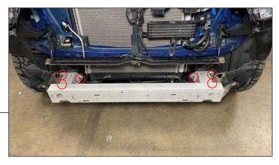
Remove (6) 14mm nuts from the aluminum vehicle bumper, and remove the bumper from the vehicle.
