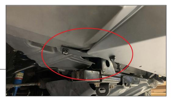
Fit the original bumper cover onto the vehicle around the new steel bumper. Secure the bumper to the vehicle using the original mounting hardware. Install the included brackets to the end bolt holes on the new bumper using the included M10 hardware. Then, insert the provided M10 hardware through the hole in the bottom of the bumper/fender liner, and secure the panels together on each side.
