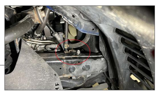
Power Steering Cooler Relocation (cont.): Through the RH side wheel well, remove the rubber liner covering the engine bay components. Unbolt the power steering cooler line from the frame. Then, fit the (1) line bracket between the cooler line and the vehicle frame. Use the original 12mm bolt to secure the bracket to the frame, and the included (1) M8 bolt, (2) M8 flat washers, and (1) M8 lock nut through the cooler line bracket.
