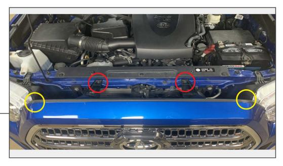
Remove grille from vehicle by removing (2) 10mm bolts, and removing (2) push clips. Lift grille away from vehicle.
