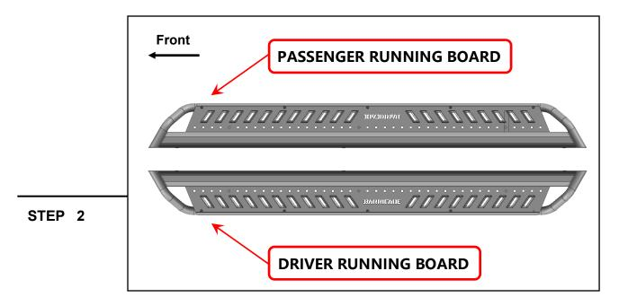
Identify each running board by identifier on the front. Notice: "D" for Driver/Left Side; "P" for Passenger/Right Side.
