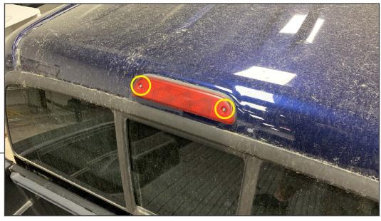
Remove (2) T-20 Torx screws from the vehicle third brake light.
