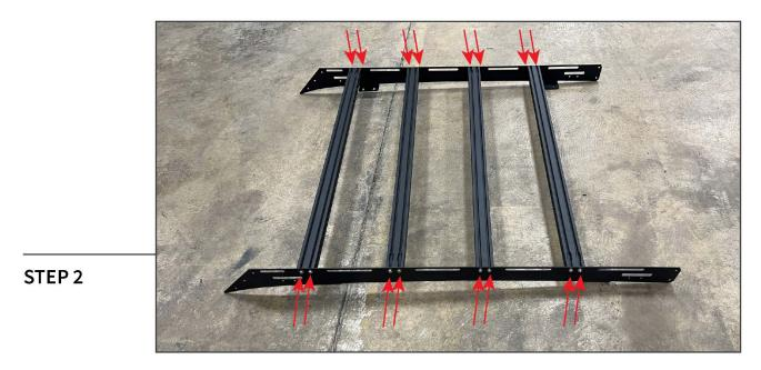
Fit the (4) cross bars between the LH and RH side rails. Then, secure the cross bars to both side rails using (16) M8 x 25mm bolts, (16) M8 lock washers, (16) M8 flat washers. Tighten evenly until secure.
