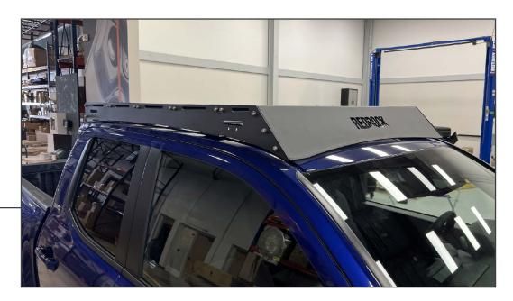
Utilize the remaining M8 eyelets and threaded inserts to add tie down points to the cross bar T-Slot system. Ensure all hardware is fully tightened.
