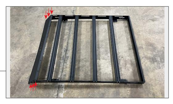
Fit the (1) front panel between the front of the side rails. Then, secure the front panel to the side rails using (6) M8 x 25mm bolts, (6) M8 lock washers, (12) M8 flat washers, and (6) M8 nuts. Tighten evenly until secure.
