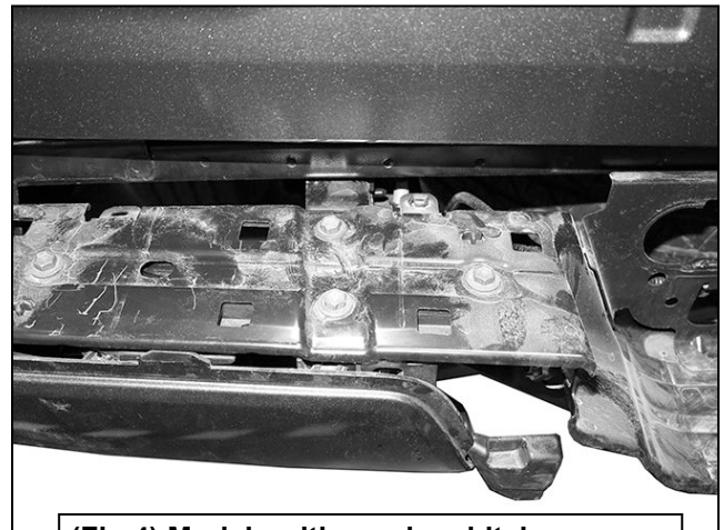
(Fig 4) Models with receiver hitch, remove the hex bolts attaching top of bumper
