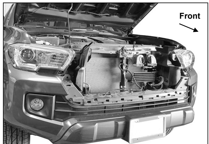
(Fig 2) Remove grille, air dam from below bumper and license plate. Remove plastic bumper cover
