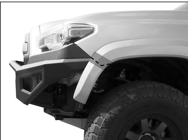
(Fig 17) Cut fender flare to match end of Bumper
