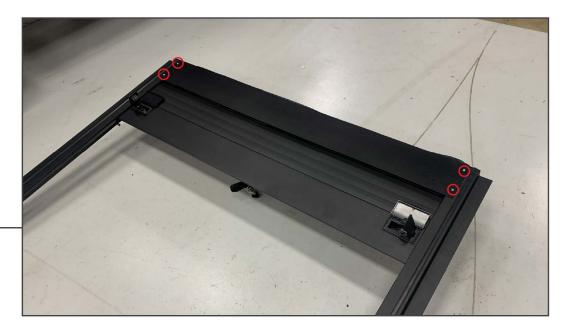
Install the upper cover panel to the tonneau cover assembly using (4) M6 x 10mm Torx bolts.
