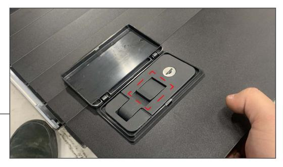
Lay out and identify all components. Place the tonneau cover assembly and the (2) side rails on a suitable working surface for assembly. Begin by unlatching the tonneau cover by pressing the release button on both sides.
