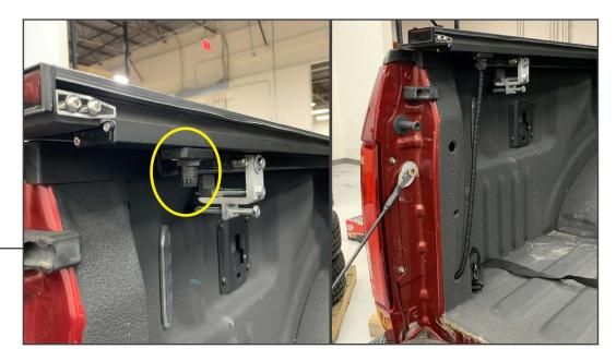
Install the rear drain tube to the side rail using an adjustable wrench, but do not over tighten. Feed the drain tube into the side rail approximately 1"-1.5". Secure the drain tube into place using the threaded cap. Route the cap drain tube through a suitable hole in the side of the bed.
