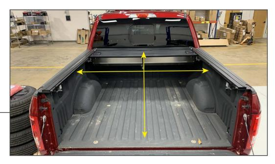
Install the (1) rear cross bar to the rear most portion of the side rails This will assist in alignment to the vehicle.
