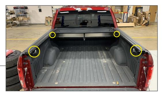
Adjust the side rails to fit flush to the bed sides. Once adjusted, tighten the clamps securing the side rails to the bed side until secure. Remove the rear cross bar once all clamps are tight.
